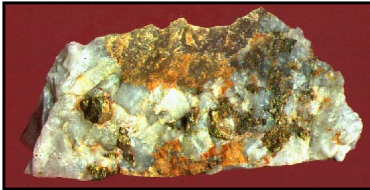
Pyrite in quartz with albitite and chlorite alteration
