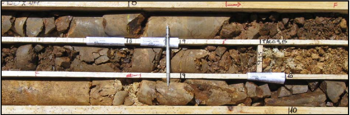
Highly altered and fractured drill core with breccia, veinlets, limonitic fractures (post- pyrite) and FeOx in fractures and a sandstone host rock
