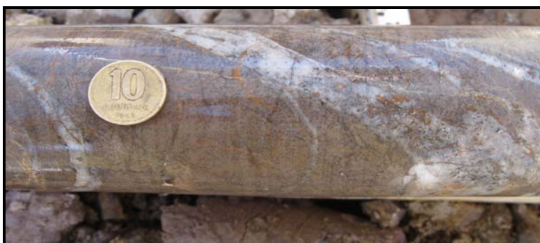
Drill core with quartz veins-veinlets, limonitic fractures (post- pyrite), FeOx in fractures and sandstone host rock
